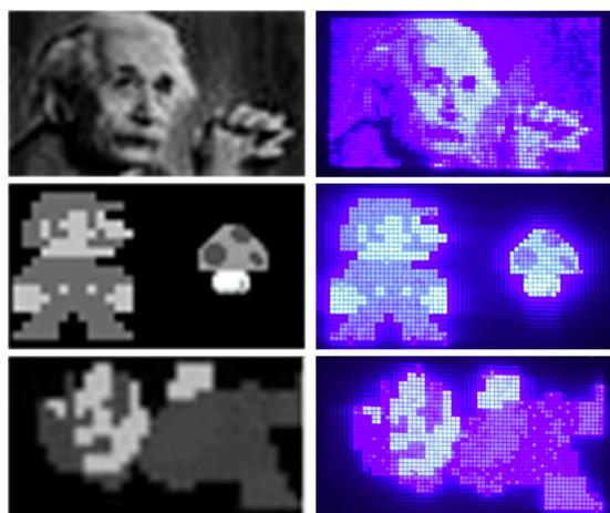
Fig. 19. Source files (left) and its corresponding display images (right) shown in the single color blue micro display system [25, 26].
