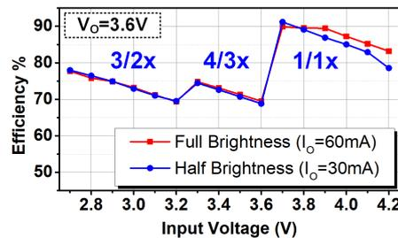
Fig. 16. Measured efficiency of hybrid voltage regulator versus input voltages [25].
