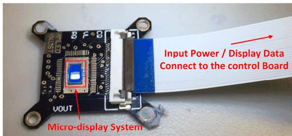
Fig. 14. PCB test board of AMLED display system with flexible cable.
