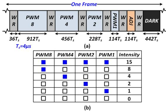
Fig. 9. (a) timing diagram of one display frame; (b) pixel intensity control with 4-bit PWM selection.
