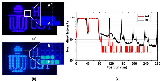
Fig. 18. Displayed and zoomed-in pattern of (a) AMLED array with silicon growth substrate removal; (b) AMLED array with conventional sapphire growth substrate; (c) Normalized intensity profiles along AA' and BB' [26].
