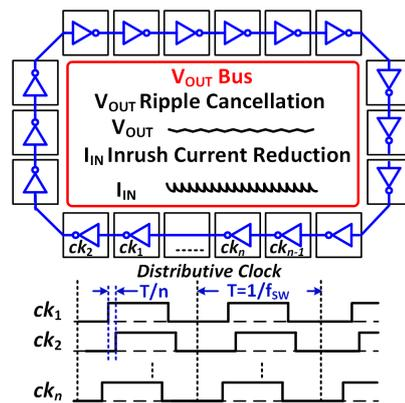
Fig. 4. Multiphase interleaving with distributive clock scheme.
