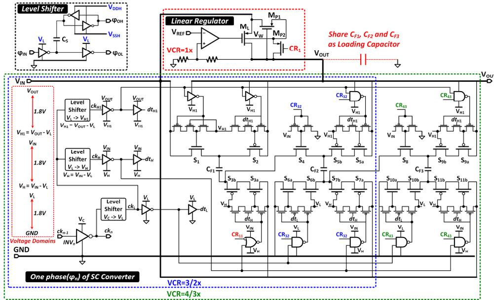
Fig. 7. Transistor level implementation of linear regulator and one power cell (phase-n), including level shifters.
