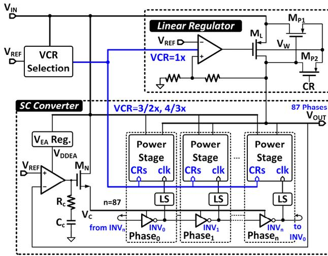
Fig. 5. System diagram of proposed integrated hybrid voltage regulator.
