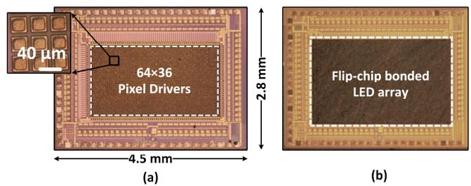
Fig. 12. (a) The micrograph of the PAD after additional Ti/Cu bilayer on silicon driving chip; (b) The integrated display system after the AMLED array chip bonded on the silicon driving chip using flip-chip packing [26].
