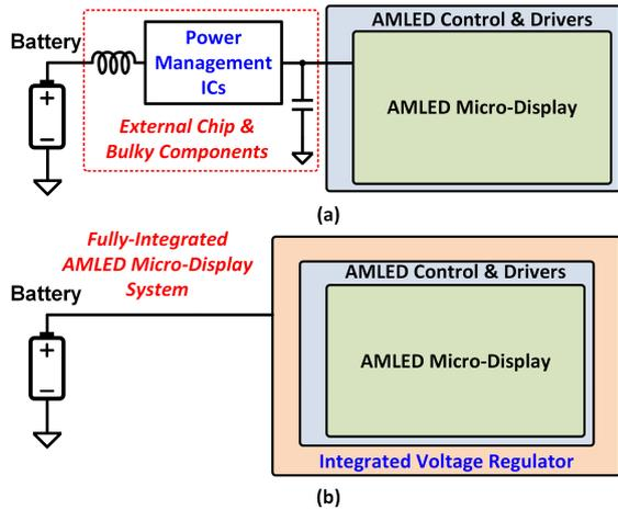
Fig. 1. (a) Conventional AMLED micro-display powered by external power management ICs; (b) Proposed fully-integrated AMLED Micro-display system with integrated voltage regulator.
