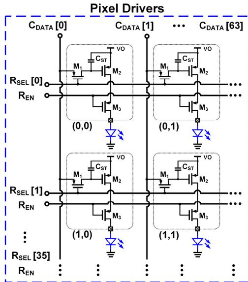
Fig. 8. Simplified schematic of pixel drivers.
