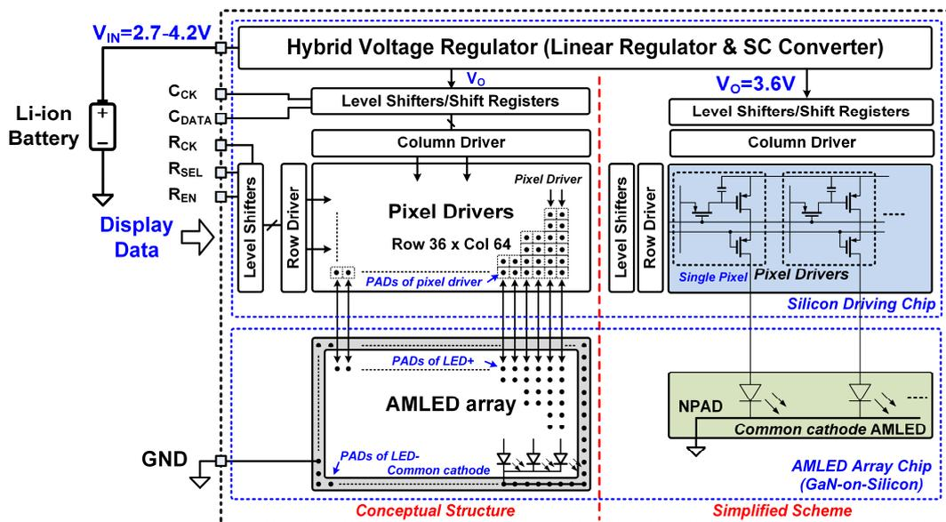
Fig. 2. The conceptual structure (left) and simplified scheme (right) of proposed micro-display system.
