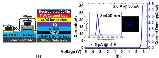
Fig. 10. (a) Vertical structure of AMLED fabrication layer; (b) I-V curve of one LED pixel [26].
