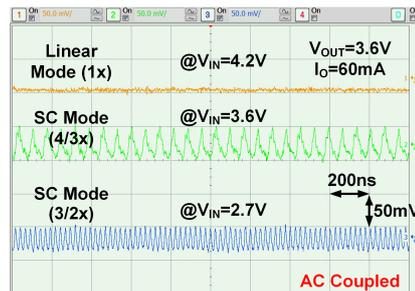
Fig. 15. Measured steady-state output voltage and voltage ripple versus  $I_O$  and  $V_{IN}$  [25].
