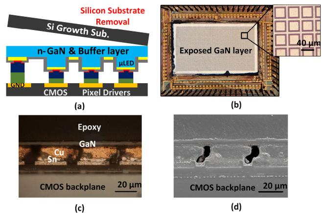
Fig. 13. (a) Silicon substrate removal process; (b) micrograph of the integrated chip after silicon substrate removal; (c), (d) micrograph and SEM image of the vertical structure of the bonding package [26].
