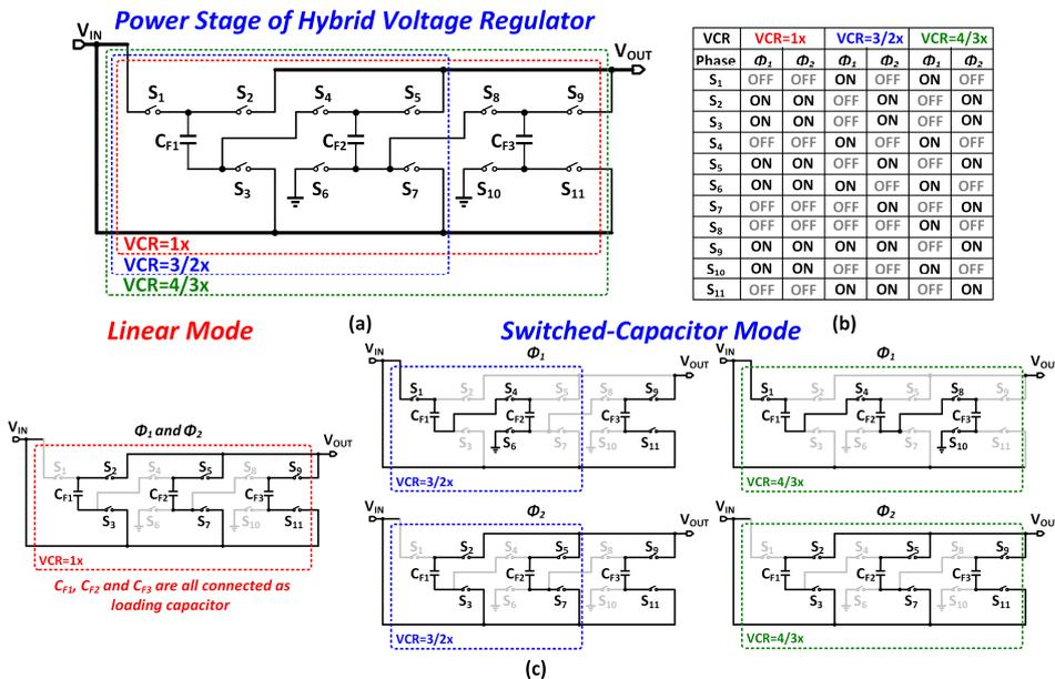
Fig. 6. (a) Schematic of power stage, (b) tabulated switches status in 3 VCRs, and (c) phase-by-phase working principles of 3 VCRs.
