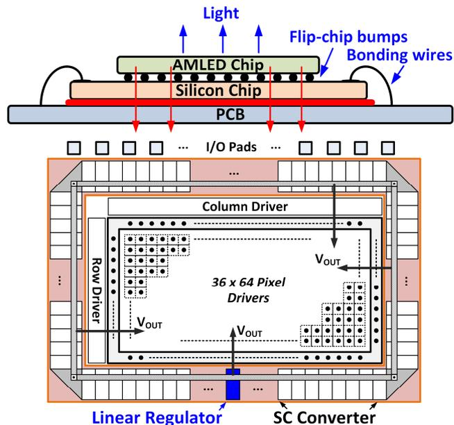
Fig. 3. The vertical structure of the system and the layout floorplan of the silicon driving chip.
