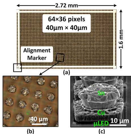
Fig. 11. (a) Micrograph of the AMLED array chip; (b) Micrograph of the Cu/Sn bumps on the top of AMLED array chip; (c) SEM photo of Cu/Sn bumps [21], [26].
