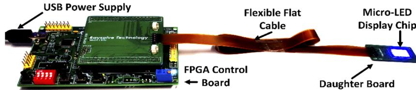
**Fig. 7.** Setup of the micro-LED display system operating in a high-brightness environment.
