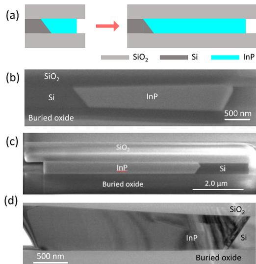
Fig. 3. (a) Schematic showing the growth of micrometer-scale InP on SOI using the “lateral ART” method. (b) Cross-sectional SEM image of 3.0  $\mu\text{m}$  wide InP grown on SOI. (c) Cross-sectional SEM image of 6.0  $\mu\text{m}$  wide InP grown on SOI. (d) Cross-sectional TEM image of micrometer-scale InP grown on SOI.
