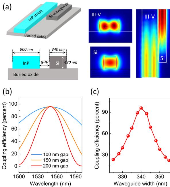
Fig. 6. (a) 3D schematic of laser with directional coupler, mode profiles inside the III-V and Si waveguides, and 2D field exchange image between the laser and Si strip waveguide for the “lateral ART” method. (b) Coupling efficiency at various wavelength for coupling gap is 100 nm, 150 nm and 200 nm. (c) The evolution of coupling efficiency in relation to the width of the Si rib waveguide. The gap is set as 100 nm.
