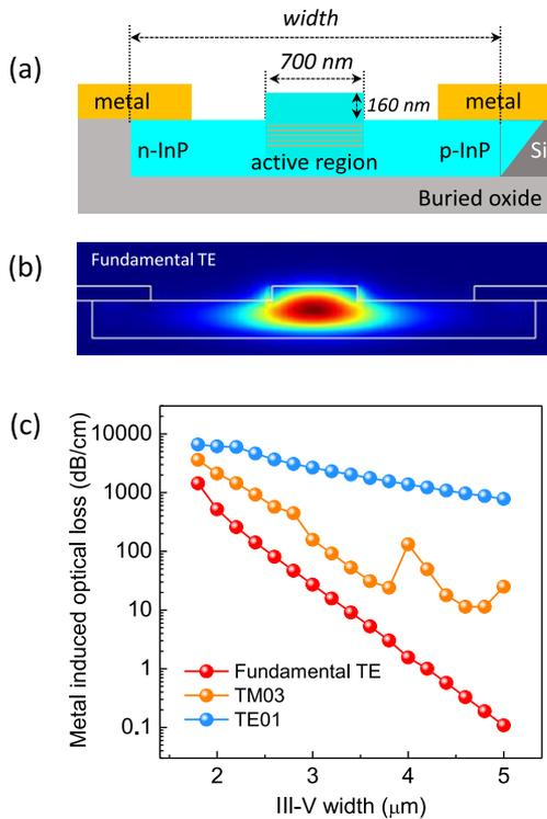
Fig. 10. (a) Schematic showing the design and simulation structure of electrically driven lasers grown on SOI using the “lateral ART” method. The flat (001)-oriented quantum wells are regrown on the InP/SOI templates. (b) Mode profile of the fundamental TE mode with an III-V width of  $3.5 \mu\text{m}$ . (c) Calculated metal-induced propagation loss of the modes supported inside the InP waveguide.
