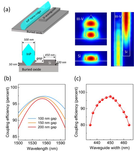
Fig. 5. (a) Coupling scheme, mode profiles, and field exchange image between the III-V laser and Si rib waveguide for the “vertical ART” method. (b) Coupling efficiency versus wavelength at varied coupling gap. (c) The evolution of coupling efficiency in relation to the width of the Si rib waveguide. The gap is set as  $100\ \text{nm}$ .
