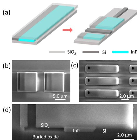
Fig. 4. (a) Schematic showing the growth of InP segments on SOI. (b) SEM image of 10  $\mu\text{m}$  long InP segments grown on SOI. (c) SEM image of 2.0  $\mu\text{m}$  long InP segments grown on SOI. (d) Cross-sectional SEM image of InP segments grown on SOI.
