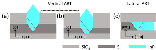
Fig. 1. (a) Schematic showing the growth of InP on V-grooved SOI using the “vertical ART” method. (b) Schematic showing the growth of InP on 220 nm SOI using the “vertical ART” method. (c) Schematic showing the growth of InP on SOI using the “lateral ART” method. The red dotted lines denote the confinement of crystalline defects at the III-V/Si interface and the block of defects by the oxide spacers.
