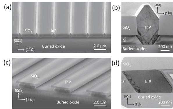
Fig. 2. (a) Tilted-view SEM image of InP nano-ridges grown on SOI using the “vertical ART” method. (b) Cross-sectional TEM image of one InP nano-ridge. (c) Tilted-view SEM image of InP grown on SOI using the “lateral ART” method. (d) Cross-sectional TEM image of InP grown laterally on SOI.
