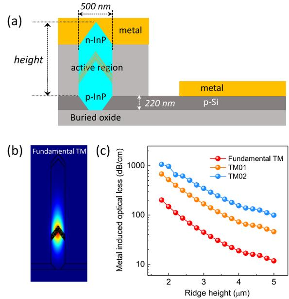
Fig. 9. (a) Schematic showing the design and simulation structure of electrically driven lasers grown on SOI using the “vertical ART” method. (b) Mode profile of the fundamental TM mode with a ridge height of 4.0  $\mu\text{m}$ . (c) Calculated metal-induced propagation loss of the modes supported inside the InP waveguide.
