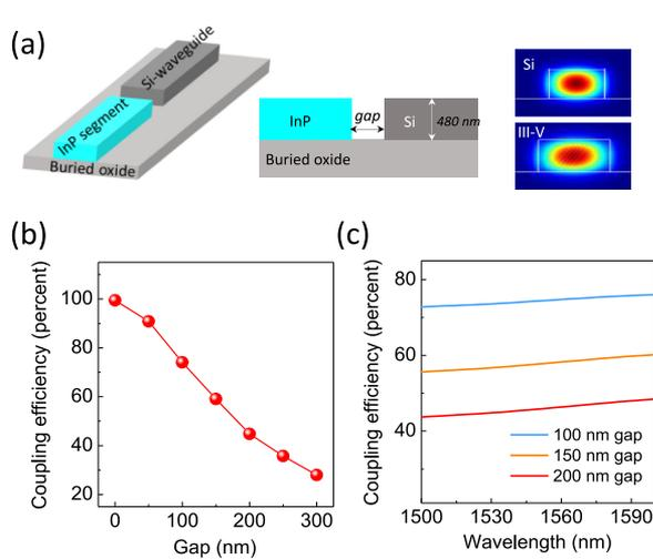
Fig. 8. (a) Butt-coupling strategy and cross-sectional view of III-V laser mode and Si waveguide mode for the “lateral ART” method. (b) Coupling efficiency versus coupling gap at 1550 nm. (c) Coupling efficiency as the function of wavelength at different coupling gap.
