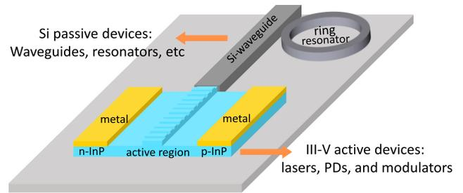
Fig. 11. Schematic illustrating the design of III-V active devices grown on SOI and seamlessly interfaced with Si-based passive components.
