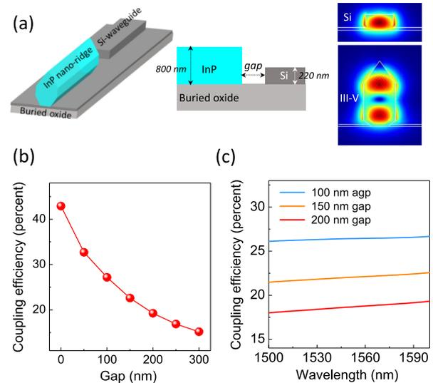
Fig. 7. (a) butt-coupling strategy and III-V laser mode and Si waveguide mode for the “vertical ART” method. (b) Coupling efficiency at 1550 nm for varied coupling gap. (c) Coupling efficiency versus wavelength at various coupling gap.
