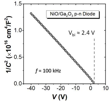
Fig. 7.  $1/C^2$  plot for the NiO/ $\beta$ -Ga<sub>2</sub>O<sub>3</sub> heterojunction p-n diode. The  $V_{bi}$  is extracted to be  $\sim 2.4$  V.
