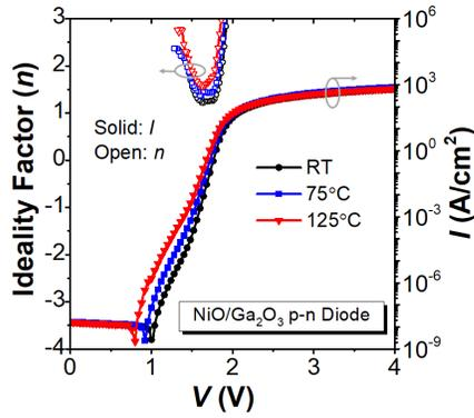
Fig. 4. Temperature dependent forward  $I$ - $V$  characteristics and ideality factors of the NiO/ $\beta$ -Ga<sub>2</sub>O<sub>3</sub> heterojunction p-n diode.
