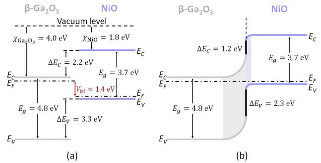
Fig. 8. The (a) theoretically estimated and (b) experimental schematic energy band diagrams of the NiO/ $\beta$ -Ga<sub>2</sub>O<sub>3</sub> heterojunction.
