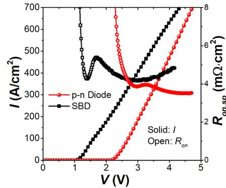
Fig. 3. Comparison of the forward  $I$ - $V$  curves for the fabricated NiO/ $\beta$ -Ga<sub>2</sub>O<sub>3</sub> heterojunction p-n diodes and Ni/ $\beta$ -Ga<sub>2</sub>O<sub>3</sub> SBDs in a linear scale.
