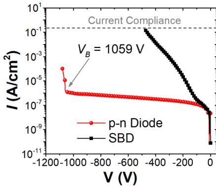
Fig. 5. Comparison of the breakdown characteristics for the fabricated vertical NiO/ $\beta$ -Ga<sub>2</sub>O<sub>3</sub> heterojunction p-n diode and Ni/ $\beta$ -Ga<sub>2</sub>O<sub>3</sub> SBD.
