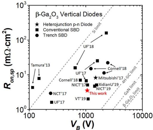
Fig. 6. Benchmark of  $R_{on,sp}$  vs.  $V_B$  of NiO/ $\beta$ -Ga<sub>2</sub>O<sub>3</sub> heterojunction diodes in this work and the previously reported vertical  $\beta$ -Ga<sub>2</sub>O<sub>3</sub> diodes.
