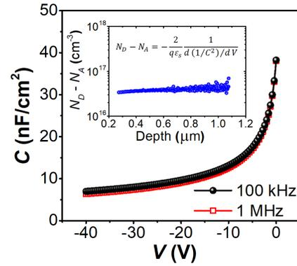
Fig. 2.  $C$ - $V$  measurement performed on the fabricated Ni/ $\beta$ -Ga<sub>2</sub>O<sub>3</sub> SBDs at 100 kHz and 1 MHz. Inset: Net doping concentration ( $N_D - N_A$ ) in the epitaxial  $\beta$ -Ga<sub>2</sub>O<sub>3</sub> drift layer extracted from the  $C$ - $V$  measurement.
