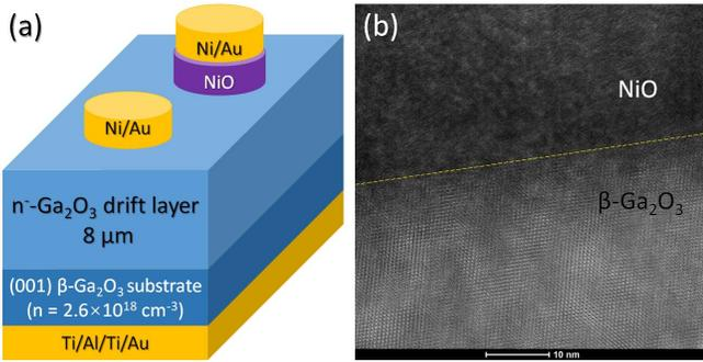
Fig. 1. (a) Schematic device structures of the vertical NiO/ $\beta$ -Ga<sub>2</sub>O<sub>3</sub> heterojunction p-n diode and the Ni/ $\beta$ -Ga<sub>2</sub>O<sub>3</sub> SBD fabricated on a bulk  $\beta$ -Ga<sub>2</sub>O<sub>3</sub> substrate, (b) cross sectional TEM image showing the hetero-interface between NiO and  $\beta$ -Ga<sub>2</sub>O<sub>3</sub>.
