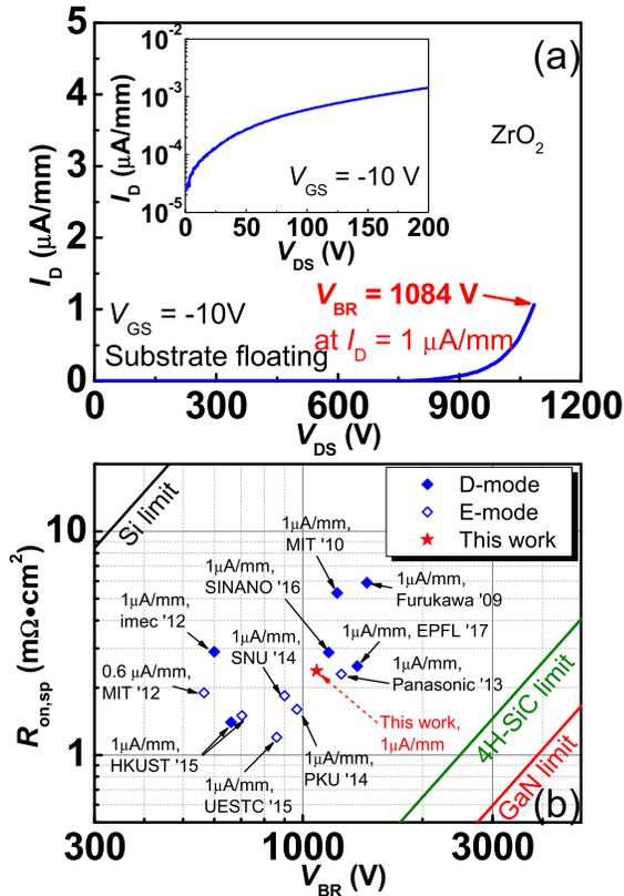
Fig. 7. (a) OFF-state drain leakage current versus drain bias. Inset: semilog plot of  $I_{DS}$  for  $V_{DS}$  under 200 V. (b) Benchmarking of  $R_{ON,sp}$  versus  $V_{BR}$  of GaN MOSHEMTs in this paper with the state-of-the-art GaN E/D-mode (MOS)HEMTs on Si by defining  $V_{BR}$  at  $I_{OFF} \leq 1 \mu\text{A}/\text{mm}$ .
