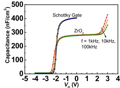
Fig. 3. Multifrequency  $C$ – $V$  characteristics of circular-shaped MOS diodes with ZrO<sub>2</sub> gate dielectric and SG.
