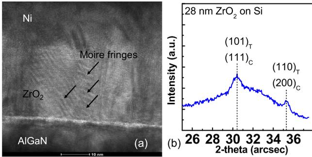
Fig. 4. (a) Cross-sectional TEM image of the ZrO<sub>2</sub> in this paper. (b) XRD pattern of 28-nm ZrO<sub>2</sub> on Si.
