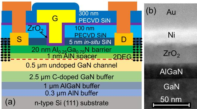
Fig. 1. (a) Cross-sectional schematic of fabricated GaN MOSHEMTs on Si with a 28-nm ZrO<sub>2</sub> gate dielectric. (b) Cross-sectional TEM image of the gate stack.
