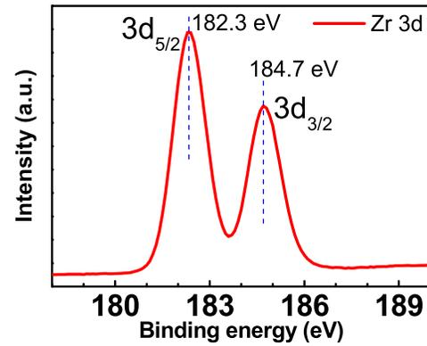
Fig. 2. XPS spectrum of Zr 3d core level of 28-nm ZrO<sub>2</sub> on AlGaIn/GaN HEMT on Si.
