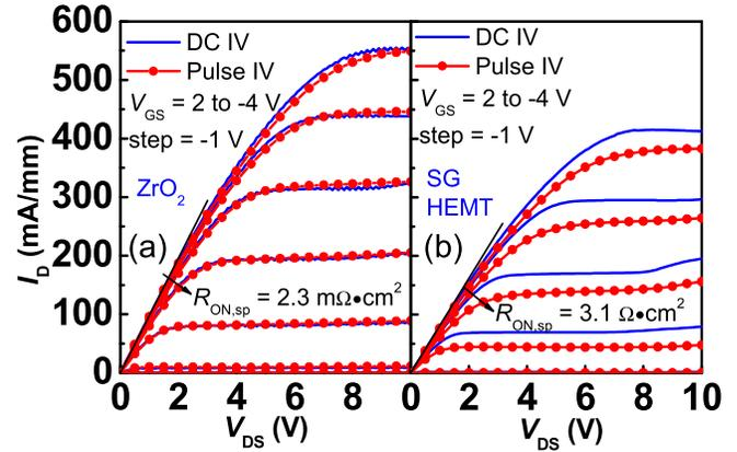
Fig. 6. Comparison of dc and gate-pulsed output characteristics of (a) ZrO<sub>2</sub>-gated MOSHEMTs and (b) SG HEMTs.
