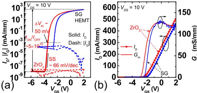
Fig. 5. Comparison of transfer characteristics of MOSHEMTs with ZrO<sub>2</sub> gate dielectric and HEMT with SG (a) in semilog scale and (b) linear scale.
