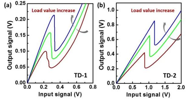
Fig. 6. (a) Output and input signal characteristic with varying load values of inverters based on (a) TD-1 (b) TD-2.
