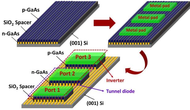
Fig. 2. Schematic and process flow of tunnel diodes and monolithically integrated inverters.
