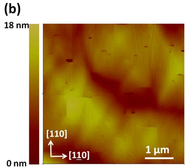
Fig. 7 (a): Tilted-view SEM image of a GaAs nanowire array with high density stacking faults; (b): AFM image of coalesced GaAs grown out of the nanowires in Fig. 7(a).
