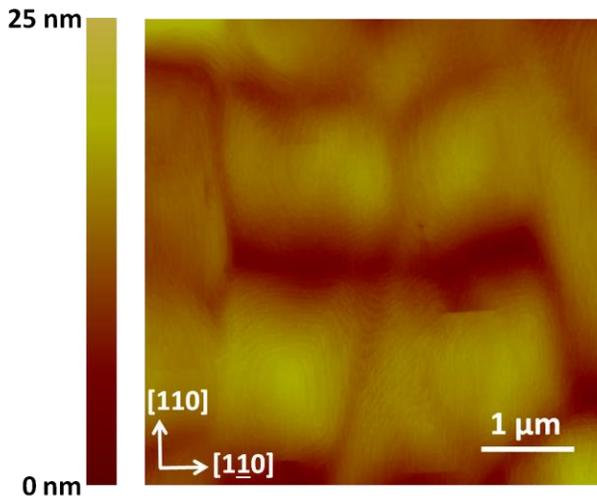
Fig. 6. AFM image of 900 nm-thick coalesced GaAs on V-grooved Si showing no antiphase-domains.
