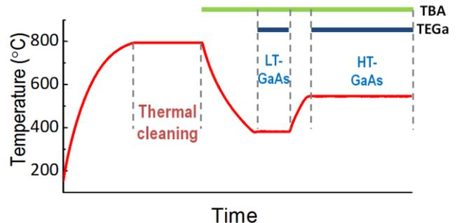
Fig.1 Schematic illustration of gas flow and temperature sequence for the planar GaAs nanowire growth on Si. (note: LT = low temperature, HT = high temperature)
