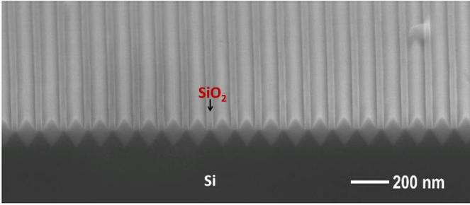
Fig.2 Tilted-view SEM image of array of planar GaAs nanowires on Si separated by SiO<sub>2</sub> sidewalls.
