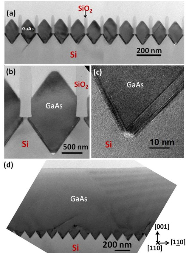
Fig.4 Cross-sectional TEM images of the planar GaAs nanowires (a)-(c) and thin films (d) taken along the [110] zone axis.
