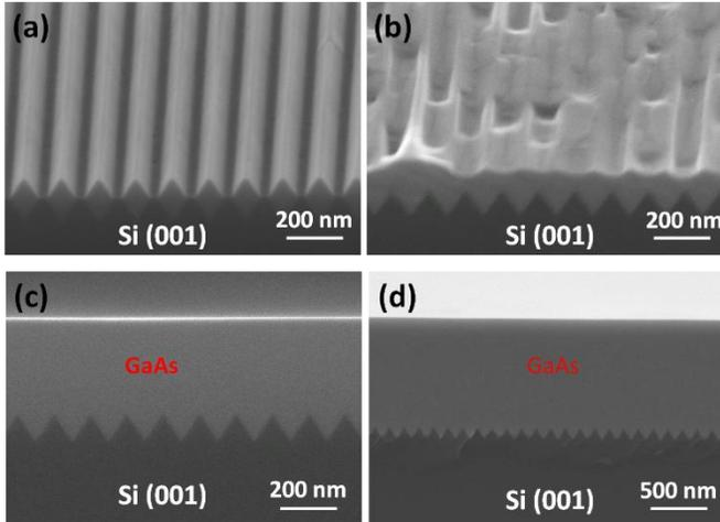
Fig.3 SEM images of the initial GaAs nanowires (a), and coalesced GaAs after 60 nm (b), 300 nm (c) and 900 nm layer overgrowth.
