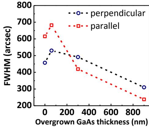
Fig. 5. XRD rocking curve FWHM from the GaAs nanowires to thin films with x-ray aligned perpendicular and parallel to the stripes.
