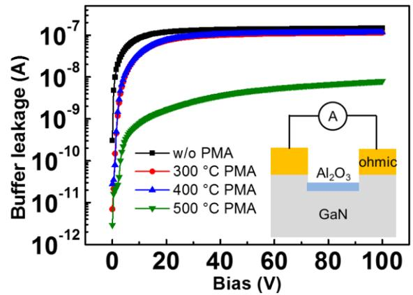
Fig. 4. Buffer leakage comparison of samples without and with various PMAs. The space between two Ohmic pads is 100  $\mu$ m.
