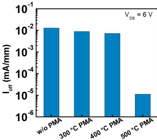
Fig. 3. Average off-state drain leakage of ten devices with same size at each PMA condition.  $I_{off}$  is determined at  $V_{GS} = -8$  V and  $V_{DS} = 6$  V.
