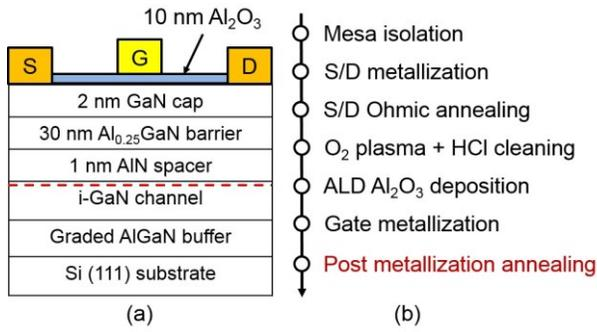
Fig. 1. (a) Schematic view and (b) process flow of fabricated Al<sub>2</sub>O<sub>3</sub>/GaN/AIGaN/GaN MOSHEMTs.
