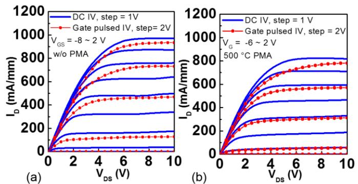
Fig. 6. DC/gate pulsed output characteristics of devices (a) without PMA and (b) with 500 °C PMA. The pulse period is 1 s and pulse width is 500  $\mu$ s. Gate pulse base voltage  $V_{GS0}$  is -8 V.
