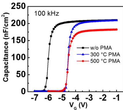
Fig. 5. Capacitance-voltage characteristics of circular MOSCAP without and with various PMAs.
