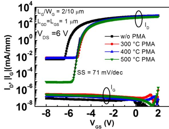
Fig. 2. Drain current and gate leakage current comparison of devices without and with various PMAs at  $V_{DS}$  of 6 V.
