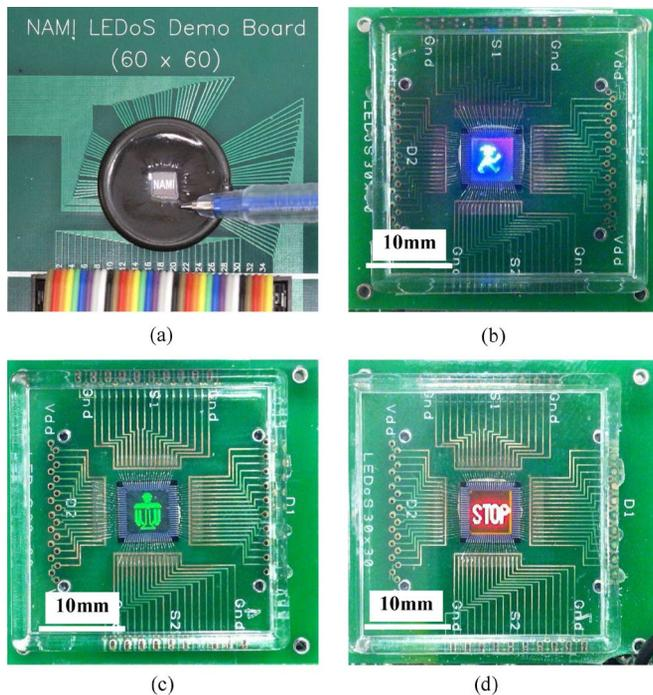
Fig. 9. Representative display results of LEDoS micro-displays with emission color of: (a) UV (b) Blue (c) Green and (d) Red.
