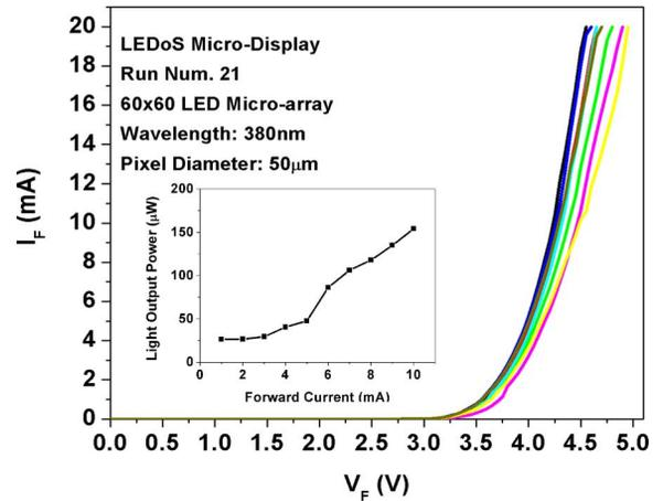
Fig. 6.  $I$ – $V$  characteristic of UV micro-LED pixels in a same row. Inset shows the  $L$ – $I$  characteristic of a representative UV micro-LED pixel.
