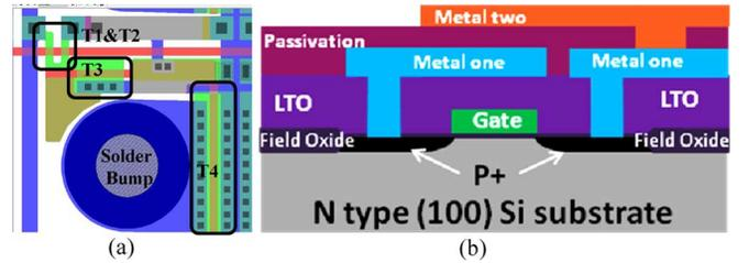
Fig. 4. (a) Layout and (b) cross-sectional view of the driving circuit.
