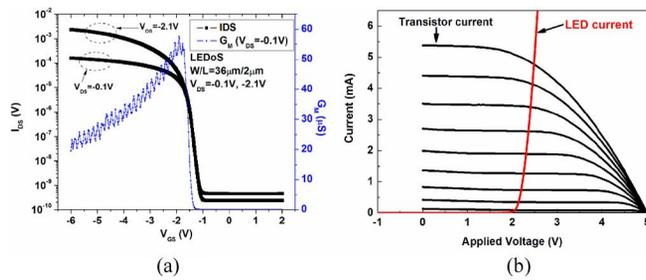
Fig. 8. (a)  $I_{D_S}$ - $V_{G_S}$  curve and (b)  $I_{D_S}$ - $V_{D_S}$  curve of the PMOS driving transistor of the current-ratio pixel circuit. Operation points of the driving transistor (Black line) and the micro-LED pixel (Red line) are also showed in (b).
