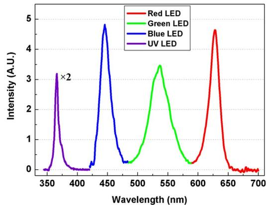
Fig. 7. Light output spectrum of the UV, Blue, Green, and Red micro-LED pixels.
