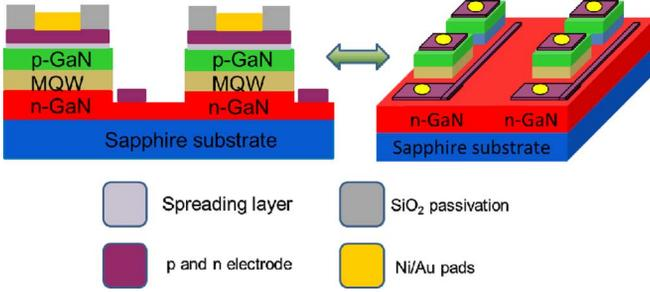
Fig. 2. Cross-sectional and 3D view of the micro-LED pixels.
