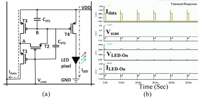
Fig. 3. (a) Schematic of the driving circuit of the active matrix substrate. The current-ratio circuit consists of four PMOS transistors and corresponds to one micro-LED pixel. (b) Spectra simulation results of the current ratio circuit.
