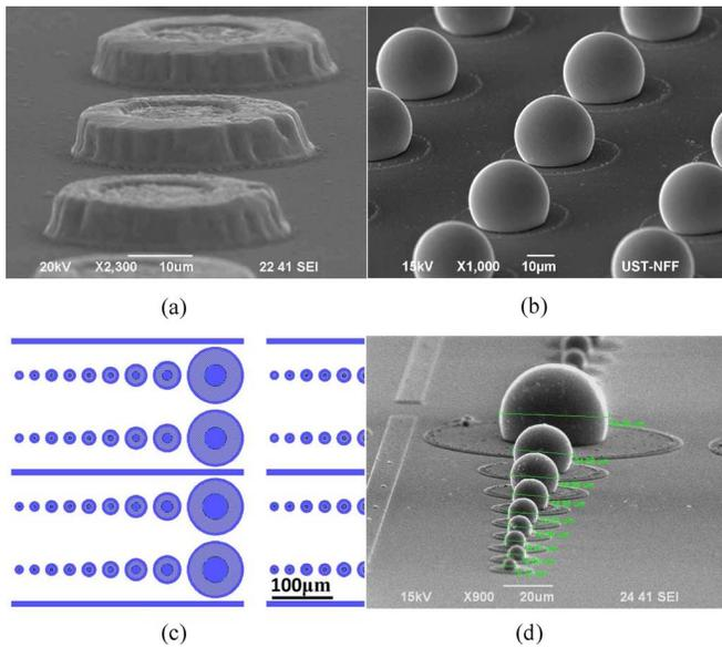
Fig. 5. (a) Illustration of a scanning electron microscopy (SEM) image of the disk-like indium pattern. (b) An SEM image of the solder bumps after the reflow process. (c) Testing structure of solder bumps. (d) Solder bumps with different diameters. The smallest one has diameter of  $5 \mu\text{m}$ .
