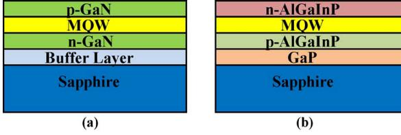
Fig. 1. (a) Epi-structure of UV, blue and green micro-LED arrays. (b) Epi-structure of red micro-LED arrays.
