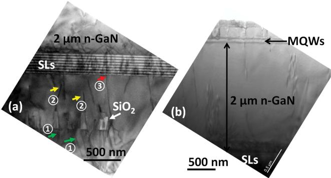
Fig. 3. Cross-sectional TEM images of the yellow LED sample (a) in the vicinity of SiO<sub>2</sub> and (b) in the 2-μm n-GaN and MQWs.
