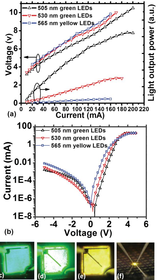
Fig. 4. (a)  $L-I-V$  characteristics of green and yellow LEDs encapsulated with silicone domes. (b)  $I-V$  characteristics. Light-emitting images of (c) 505-nm LEDs, (d) 530-nm LEDs, and (e), (f) 565-nm LEDs.
