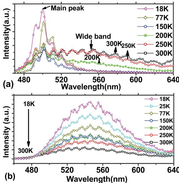
Fig. 5. Temperature-dependent PL spectra of (a) 505-nm green LEDs and (b) 565-nm yellow LEDs.
