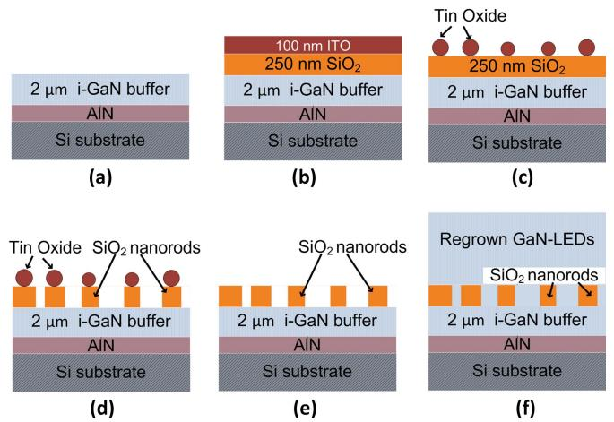
Fig. 1. Schematic diagram of the preparation procedure of GaN-based LEDs with embedded  $\text{SiO}_2$  nanorods (a) 2- $\mu\text{m}$  GaN deposition on Si. (b)  $\text{SiO}_2$  and ITO deposition. (c) ITO patterning in HCl. (d)  $\text{SiO}_2$  dry etching. (e) Dry etching mask removal. (f) Regrowth of GaN-based LEDs.
