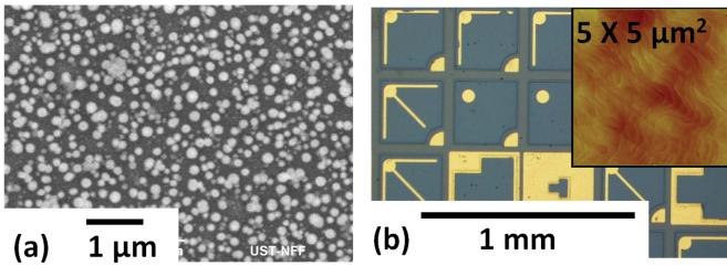
Fig. 2. (a) Planar view SEM image of SiO<sub>2</sub> nanorods on the GaN surface. (b) Microscopic image of the fabricated yellow LEDs ( $5 \times 5 \mu\text{m}^2$  AFM image of the regrown yellow LED surface).
