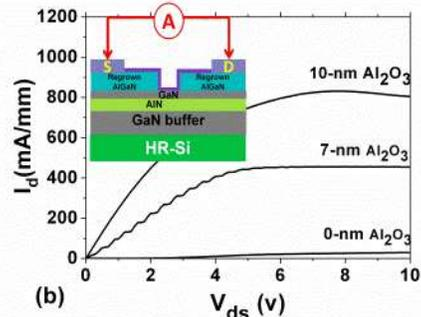
Fig. 5. DC  $I_d$ - $V_{\text{ds}}$  characteristics of transistors before gate metal deposition with different  $\text{Al}_2\text{O}_3$  thickness. Source-drain spacing is  $4.5\ \mu\text{m}$ . Inset is schematic view of the measured structure.
