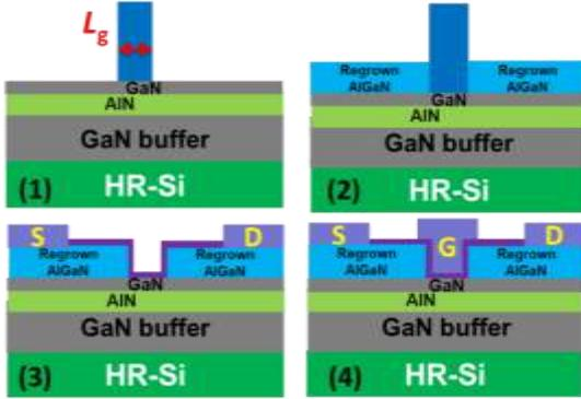
Fig. 2. Regrowth and simplified process flow of MOSHEMTs: (1) pattern with  $\text{SiO}_2$ , (2) regrowth of AlGaIn barrier layer, (3)  $\text{SiO}_2$  strip, source/drain ohmic formation and 7-nm  $\text{Al}_2\text{O}_3$  deposition, (4) gate metal deposition.
