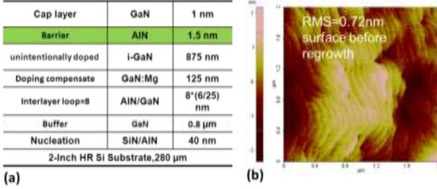
Fig. 1. (a) AlN/GaN heterostructure. (b) Surface morphology scanned by AFM.
