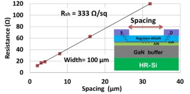
Fig. 4. TLM of the sample with regrown AlGaIn cap layer. Inset: schematic view of the measured structure.
