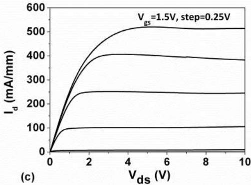
Fig. 6. (a) SEM image of the fabricated E-mode transistor with 60 °C tilt view angle. (b) Transfer and (c) DC  $I_d$ - $V_{ds}$  characteristics for AlN/GaN MOSHEMTs carried out by annealing.
