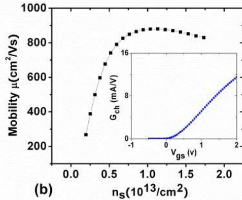
Fig. 7. (a) Plot of measured on-state resistance versus gate length ( $L_g$ ) for transistors with differing  $L_g$  and varying gate voltages. The total access region length is around  $4.3 \mu\text{m}$ . (b) Extracted channel mobility dependence on 2DEG concentration. Inset is the plot of channel conductance versus gate voltage.
