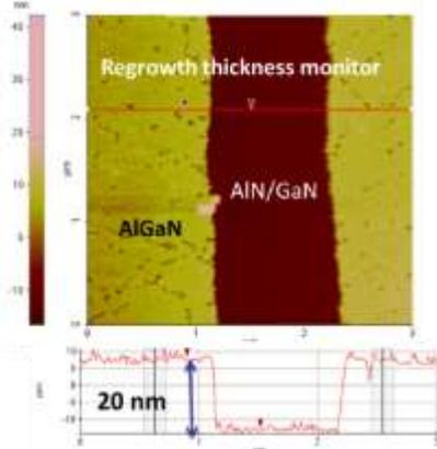
Fig. 3. AFM image of the regrowth profile in the gate region after  $\text{SiO}_2$  is removed.
