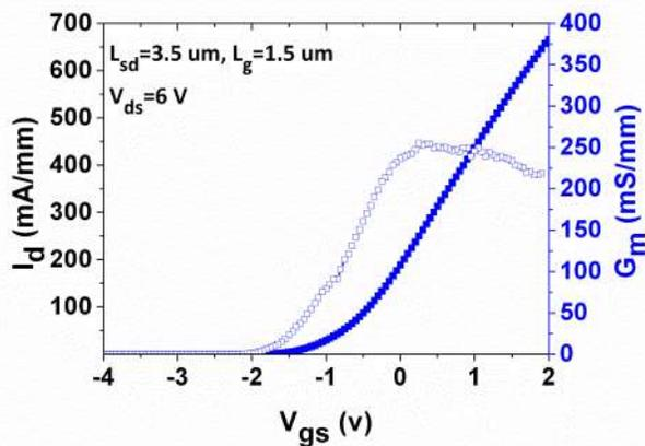
Fig. 8. DC transfer characteristics of AlN/GaN MOSHEMTs fabricated without post-gate annealing
