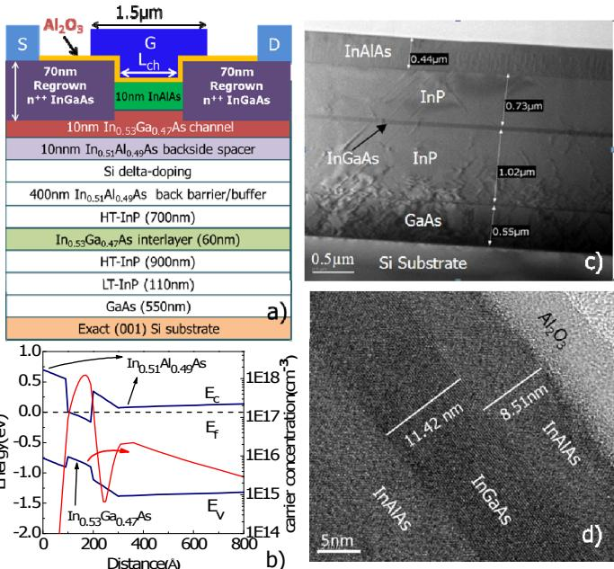
Fig.1: (a) Schematic of device with nominal layer thicknesses (LT-low temperature, HT-high temperature, note: figure is not drawn to scale), (b) Simulated band diagram and carrier distribution of the quantum well structure corresponding to Fig.1a, (c) Cross-sectional TEM image of the composite buffer layers grown on Si substrate, (d) Cross-sectional TEM image of oxide and InAlAs/InGaAs active layers with gate oxide.
