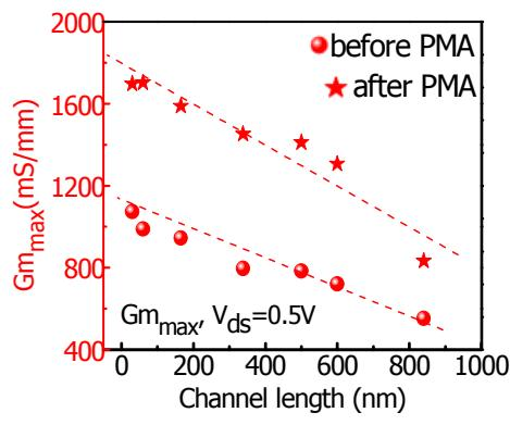
Fig.9: Peak transconductance ( $Gm_{max}$ ) measured at  $V_{ds}=0.5V$  as a function of channel length.
