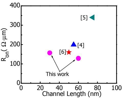
Fig.12: Comparison of  $R_{on}$  with state-of-the-art InGaAs MOSFETs
