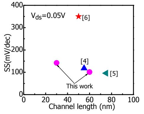
Fig.13: Comparison of SS measured at  $V_{ds}=0.05V$  with state-of-the-art InGaAs MOSFETs
