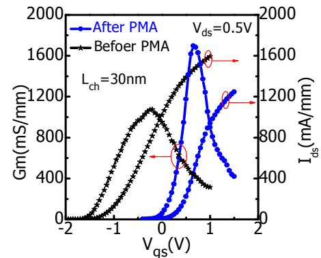
Fig.4: Transfer characteristics of a 30nm device measured with the device in Fig.2 before/after PMA.
