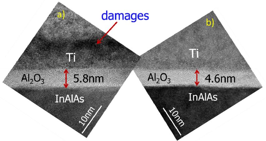
Fig.15: High-resolution cross-sectional TEM images of gate metal/oxide/InAlAs gate stacks before (a) and after (b) PMA, showing reduced oxide thickness and recovered damages from E-beam metallization, leading to abrupt and flat Ti/oxide/InAlAs interfaces.
