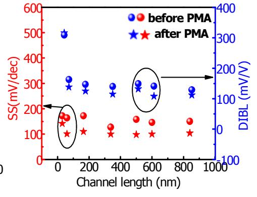
Fig.10: Subthreshold slope (SS) at  $V_{ds}=0.5V$  and drain induced barrier lowering (DIBL) as a function of channel length
