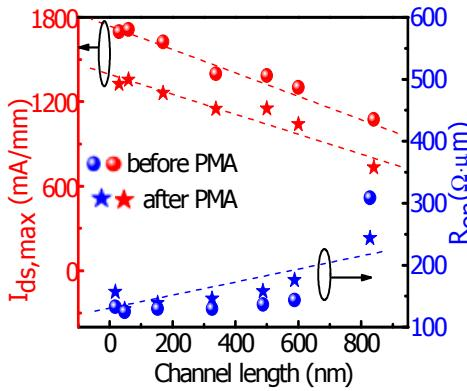
Fig.8: Maximum drain current ( $I_{ds,max}$ ) at  $V_{ds}=0.5V$  and on-resistance ( $R_{on}$ ) as a function of channel length.
