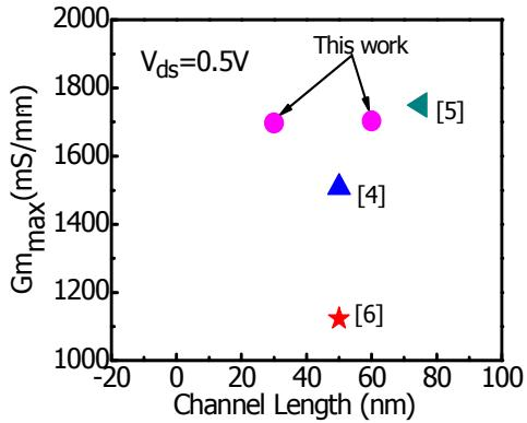
Fig.11: Comparison of  $Gm_{max}$  measured at  $V_{ds}=0.5V$  with state-of-the-art InGaAs MOSFETs
