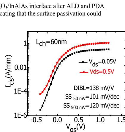
Fig.6: Transfer characteristics of a device with a  $L_{ch}$  of 60nm after PMA
