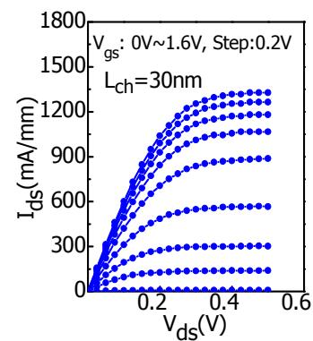
Fig.7: Output characteristics of a 30nm channel-length E-mode device after PMA
