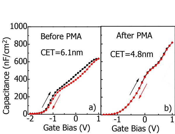
Fig.14: 1MHz C-V measurement of  $Al_2O_3/InAlAs/ InGaAs$  capacitor before and after PMA, where the gate bias was swept bi-directionally. Increased gate capacitance and greatly reduced hysteresis are obtained after PMA.
