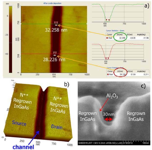
Fig.2: (a) AFM line profile of a  $L_{ch}=30$  nm device scanned after gate dielectric deposition. The channel length is defined by the regrown source/drain separation. Several positions have been measured across the channel with an average  $L_{ch}$  of 30nm. Two representative positions (red line and green line) were shown, (b) 3-dimensional AFM image corresponding to Fig.2a, (c) Cross-sectional SEM image of a  $L_{ch}=30$  nm device after whole process.
