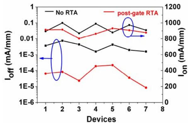
**Figure 4**  $I_{\text{on}}$  and  $I_{\text{off}}$  distribution in devices across the samples before and after post-gate RTA.
