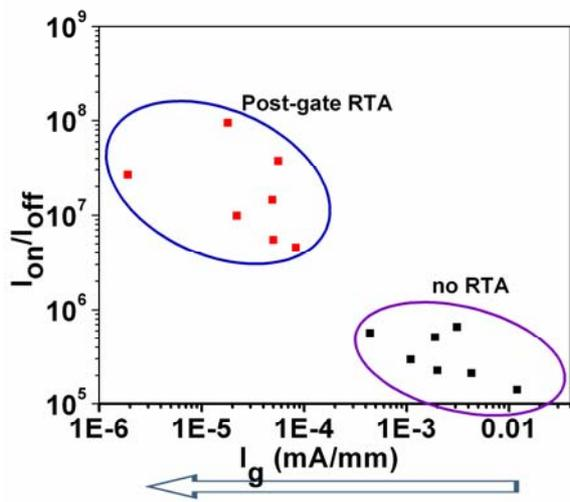
**Figure 5** Correlation between  $I_{on}/I_{off}$  and gate leakage current.  $I_g$  was measured at  $V_{gs} = -8$  V from the gate-source  $I$ - $V$  characteristics.
