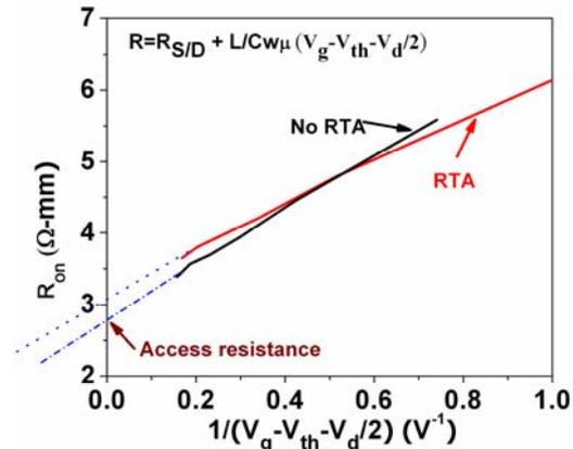
**Figure 3** Slight increase in access resistance extrapolated from on-state resistance of samples before and after post-gate RTA.
