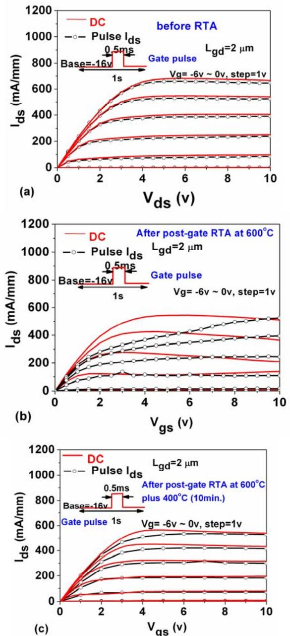
**Figure 7** Pulsed  $I$ - $V$  characteristics of samples: (a) before RTA, (b) after post-gate RTA at 600 °C, and (c) after post-gate RTA at 600 °C and another RTA at 400 °C for 10 minutes.
