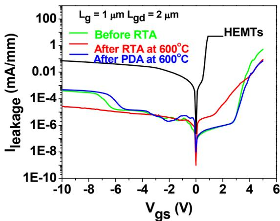
**Figure 6** Comparison of gate leakage current of samples under three different thermal treatments: before RTA, post-gate RTA, and PDA.
