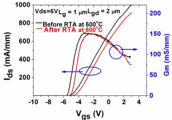
**Figure 2** Transfer characteristics (linear-scale) of samples before and after post-gate RTA.
