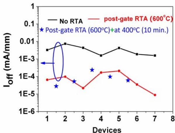
**Figure 8**  $I_{\text{off}}$  of three kinds of samples: before RTA, after post-gate RTA at 600 °C, and after post-gate RTA at 600 °C plus another RTA at 400 °C for 10 minutes.
