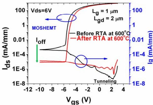
**Figure 1** Transfer characteristics (semi-log-scale) and gate current of sample before and after post-gate RTA at 600 °C.
