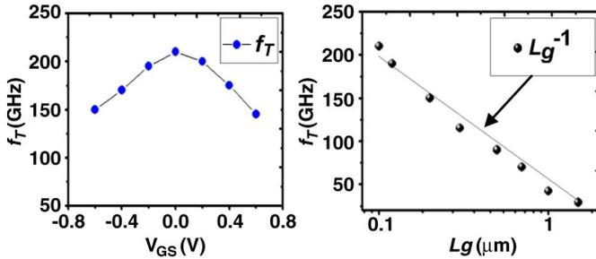
Fig. 6. Dependence of  $f_T$  on gate bias and gate length ( $L_g$ ) for our mHEMTs, where  $V_{DS}$  is fixed at 1.0 V.
