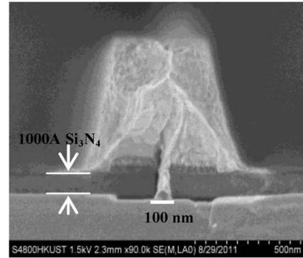
Fig. 3. Cross-sectional SEM graph of a T-shaped gate.
