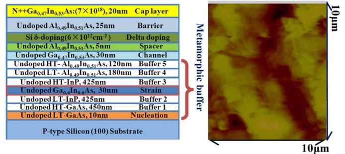
Fig. 1. Nominal structure of an mHEMT device on a Si substrate and an AFM image of  $10 \times 10 \mu\text{m}^2$  scan area of buffer structures on a Si substrate.
