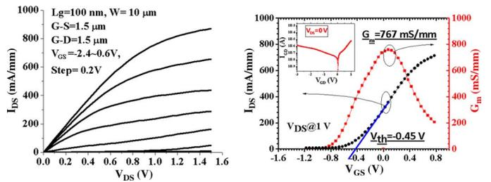
Fig. 4. DC  $IV-V$  characteristics and transfer characteristics of a  $0.1 \times 10 \mu\text{m}^2$  mHEMT.
