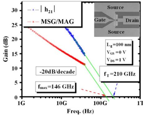
Fig. 5. Cross-sectional SEM graph and current gain MSG/MAG as a function of frequency of a  $0.1 \times 100 \mu\text{m}^2$  T-shaped gate mHEMT.
