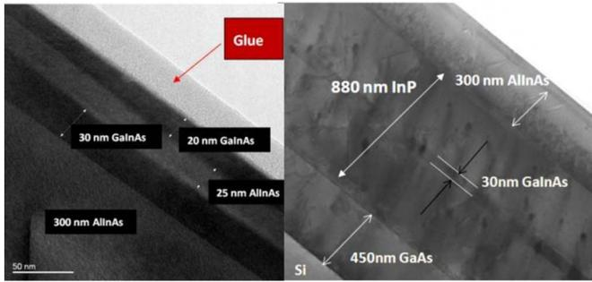
Fig. 2. TEM cross section micrograph of an mHEMT structure.
