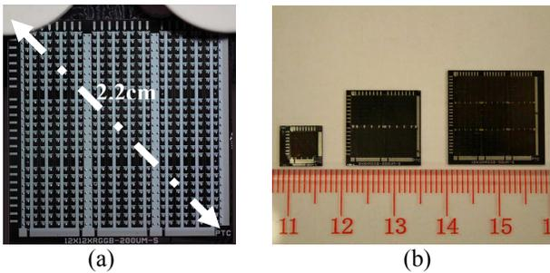
Fig.10 (a)  $24 \times 24$  active matrix substrate with solder bumps on each pixel and (b) 1, 4, and 9 modules integrated on large area active matrix substrates
