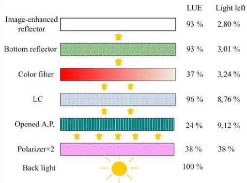
Fig.1 LCD light output based on light losses per layer [2]
