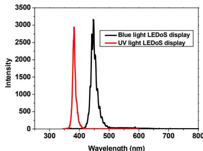
**Fig. 7** Wavelength of blue and UV LEDoS displays
