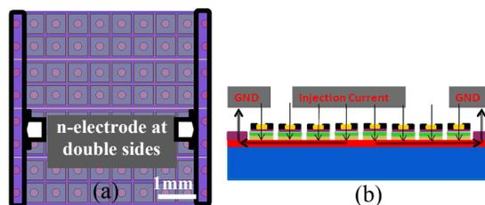
Fig. 3 (a) Layout of the 8 × 8 LED micro-array module and (b) current flow of 8 LED pixels in a row
