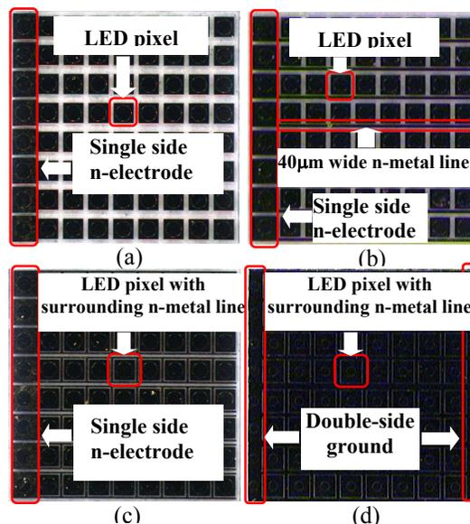
Fig.4 (a) without any optimization; (b) with 40μm-wide n-metal line; (c) with n-metal surrounding; (d) with n-metal surrounding and double-side cathodes
