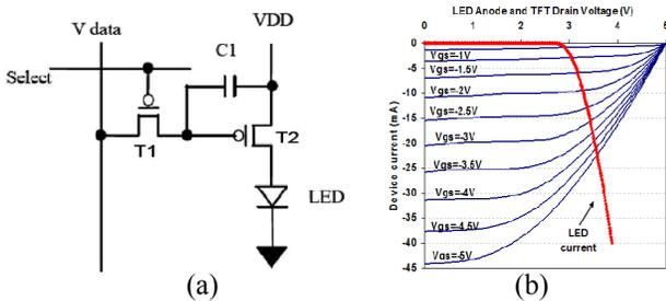
Fig. 9 (a) Schematic of LEDoS pixel circuit and (b) operation points of driving transistor and LED pixel
