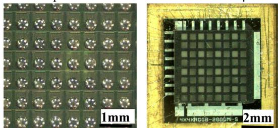
Fig.2 (a) solder bumps seating on top of active matrix substrate and (b) microscope image of LEDoS module after RGB phosphors deposition
