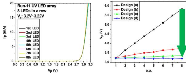
**Fig. 5** (a) I-V characteristics of 8 LEDs in the same row of double-side ground structure; (b)  $V_F$  variation of LED pixels with four designs
