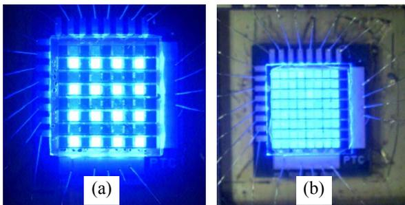
**Fig. 6** The blue light LEDoS module was (a) individually lit up and (b) fully lit up
