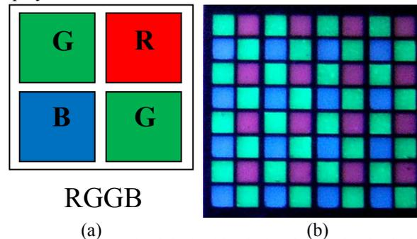
**Fig. 8** (a) One colorful pixel includes four sub-pixels in combination of RGGB and (b) a full-color display by excitation of RGB phosphors by UV LEDs
