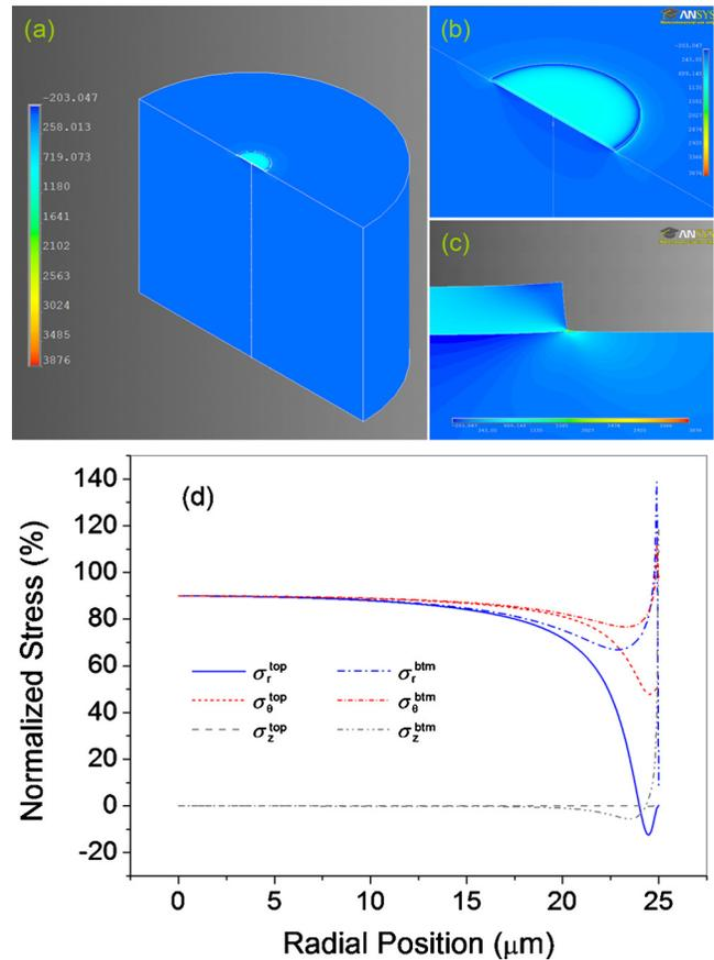
FIG. 3. (Color online) (a) Spatial distribution of  $\sigma_r$  in the GaN/Si bilayer system ( $R=25 \mu\text{m}$ ). (b) Close-up views of the stress field ( $\sigma_r$ ). (c) Stress concentration at the edge of the island. (d) Stress distribution along the radial direction at top surface and bottom interface of the coin-shaped GaN island.
