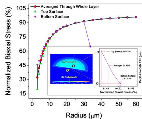
FIG. 4. (Color online) Normalized biaxial stress, from FEA, at the island center vs the island radius, where the triangles indicate the normalized stress level at top surface and bottom interface at the island center and the circles show the average stress level on the point all through the vertical axis. The inset shows one example ( $R=30 \mu\text{m}$ ) of depth dependence of relaxed stress.
