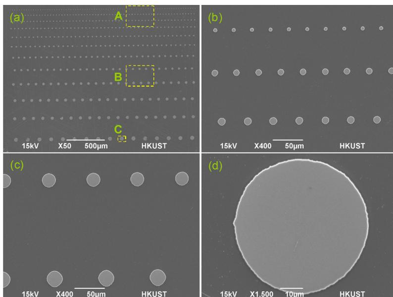
FIG. 1. (Color online) (a) Fabricated array of coin-shaped GaN islands. Close-up views at regions A, B, and C in (a) are given in (b), (c), and (d), respectively. The island radii are approximately 3, 5, and  $6\ \mu\text{m}$  in (a), 11 and  $13\ \mu\text{m}$  in (b), and  $31\ \mu\text{m}$  in (c).
