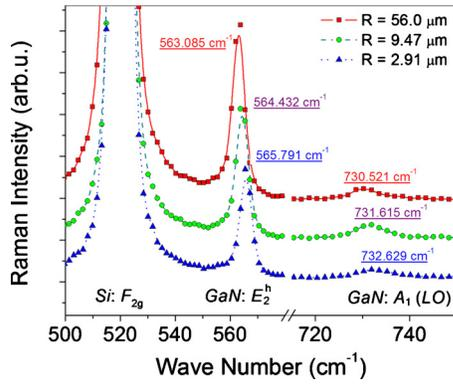
FIG. 5. (Color online) Raman spectra captured at centers of the coin-shaped islands with distinct radiuses.
