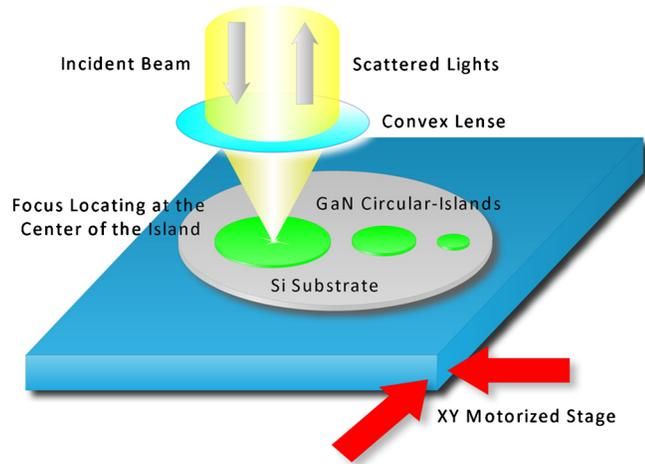
FIG. 2. (Color online) Schematic illustration of the experimental setup.
