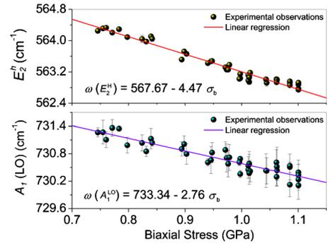
FIG. 6. (Color online) Linear relationship between observed  $E_2^H$  and  $A_1(LO)$  phonon frequencies and biaxial stress.
